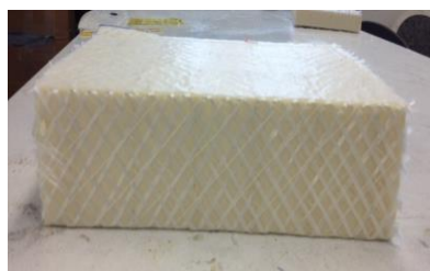
Figure 3 Type-3 Web-core foam with mat reinforcement
