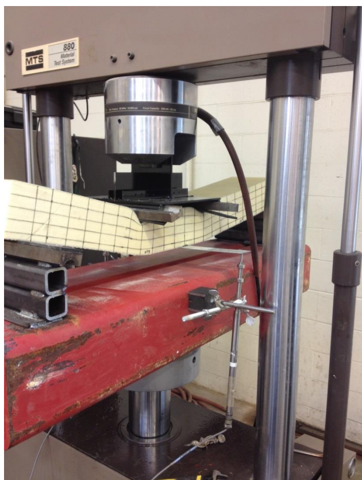
Figure 5 Shows panel deflection during the test
