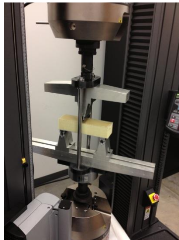
Figure 6 Flexural test setup
