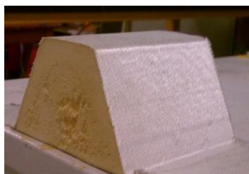
Figure 2 Type-2 Trapezoidal low density foam with mat reinforcement
