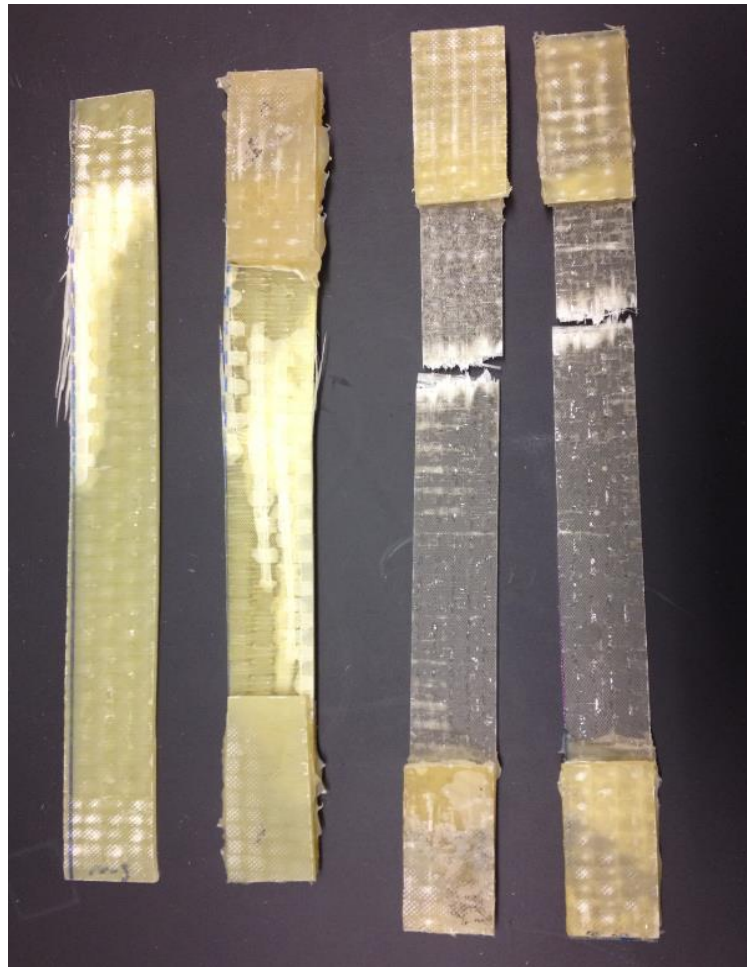
Figure 10 Tensile specimens after testing The glass fiber/PU840871 specimens (right) typically failed laterally. The glass fiber/ PU90IK01 specimens (left) typically failed by splaying of the fibers.
