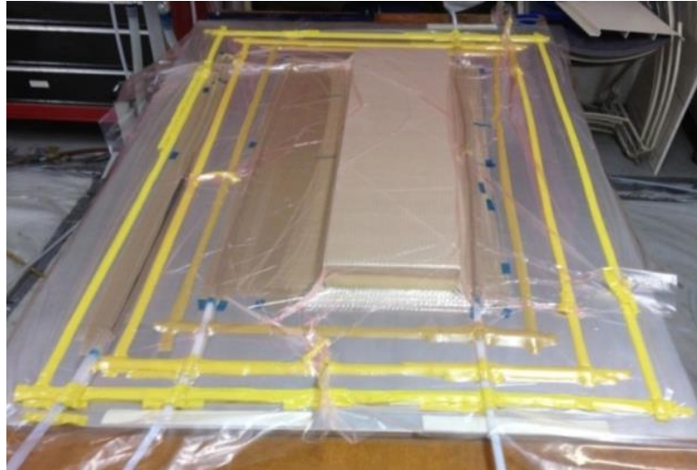
Figure 5 VARTM setup for sandwich composite
